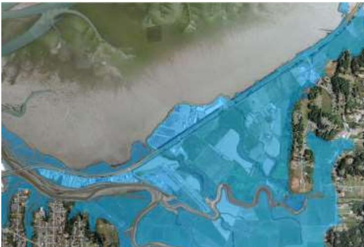
*Assuming tidal elevation is 9.99 feet (MMMW+100-year stillwater level) and that protective shoreline structures are compromised north of Airport Road, extensive flooding of south and north bound lanes.*
