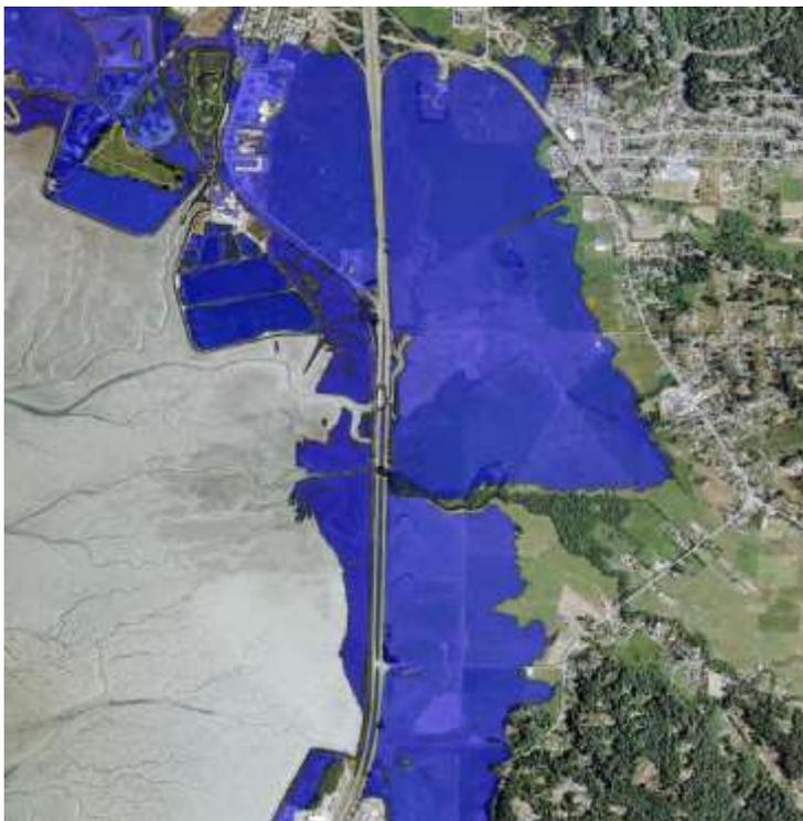
*Assuming tidal elevation is 9.38 feet (MMMW+0.5 meter sea level rise) and that protective shoreline structures are compromised, the land adjacent to the road prism is inundated to the west and east of Highway 101.*
