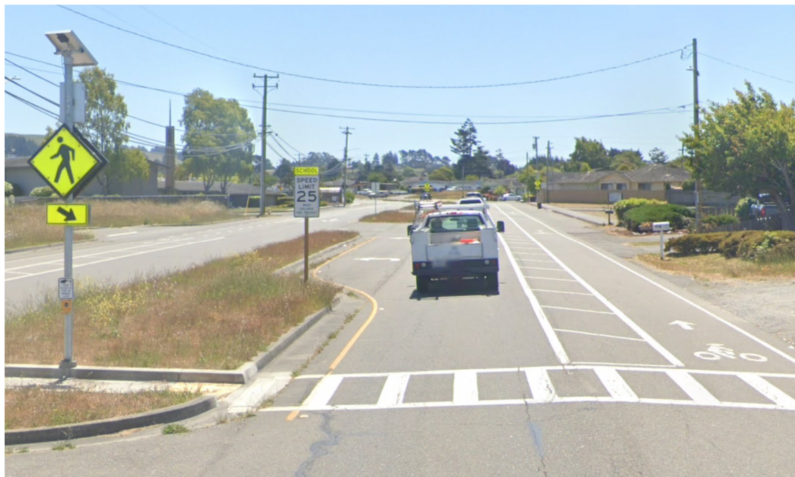
Figure 2.2 School Zone Speed Limit Sign on Ross Hill Road
