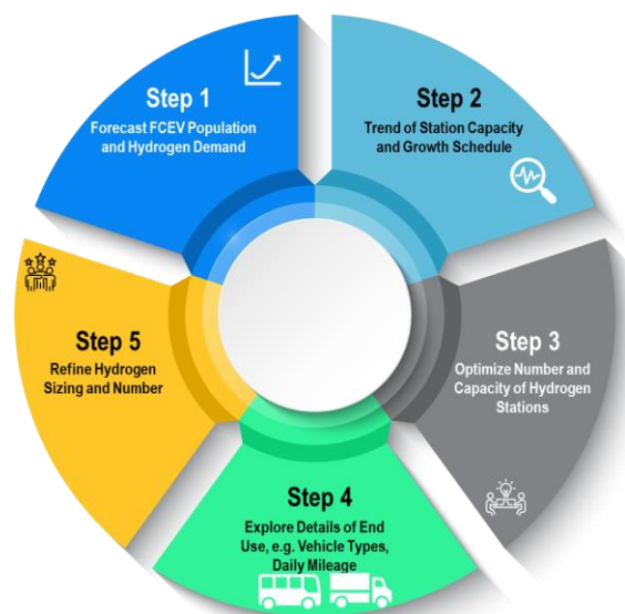
Exhibit 12. An Illustration of the Process to Estimate Number and Size of Hydrogen Stations
