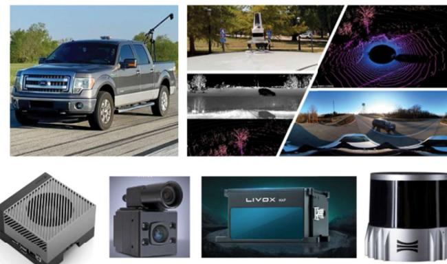
Figure 1: Examples of TEE Data Collection Sensors
