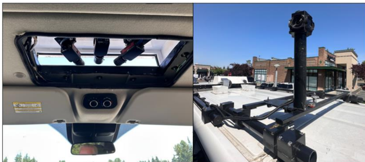
Figure 8. Forward-Facing HD+ Cameras (on the left) and LadyBug Camera (on the right).
