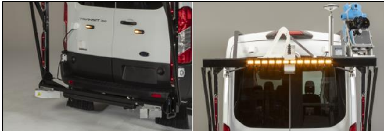
Figure 10. Inertial Profilers (Left) and Laser Camera for Pavement Imaging (Right).
